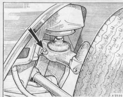
The inner pivot of the upper support arm is lubricated through the grease nipple provided on each side
