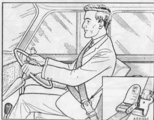
A static seat belt, showing the correct position of the buckle
